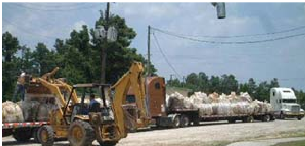
Figure 2. Loading super sacks of turkey litter and dewatered swine solids for transportation
