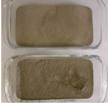
Figure 5. Potassium enriched (top) and chlorine enriched (bottom) ash.
