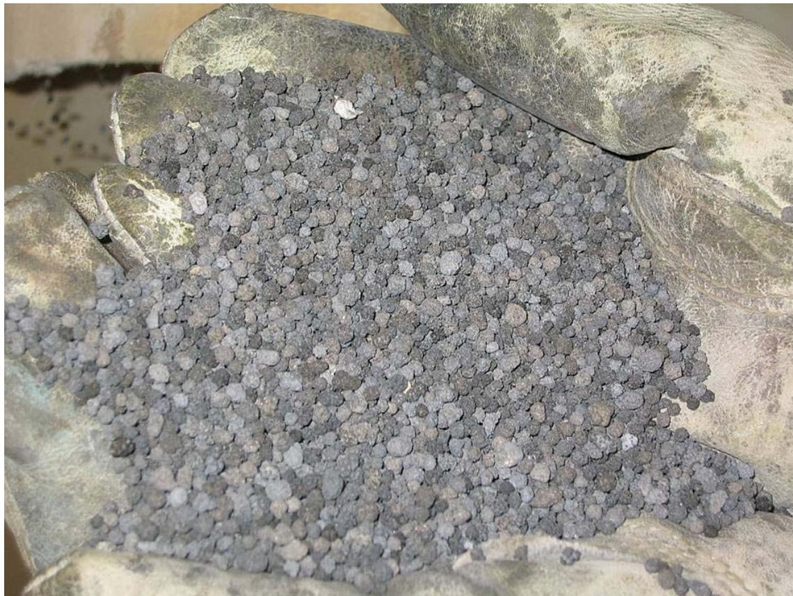
Figure 5. Fertilizer granules produced in ACT pilot plant.
