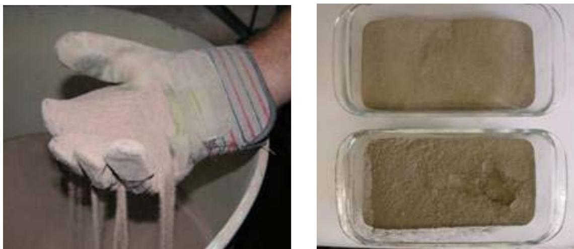
Figure 4. Cyclone ash (left and upper right) and baghouse ash (lower right).
