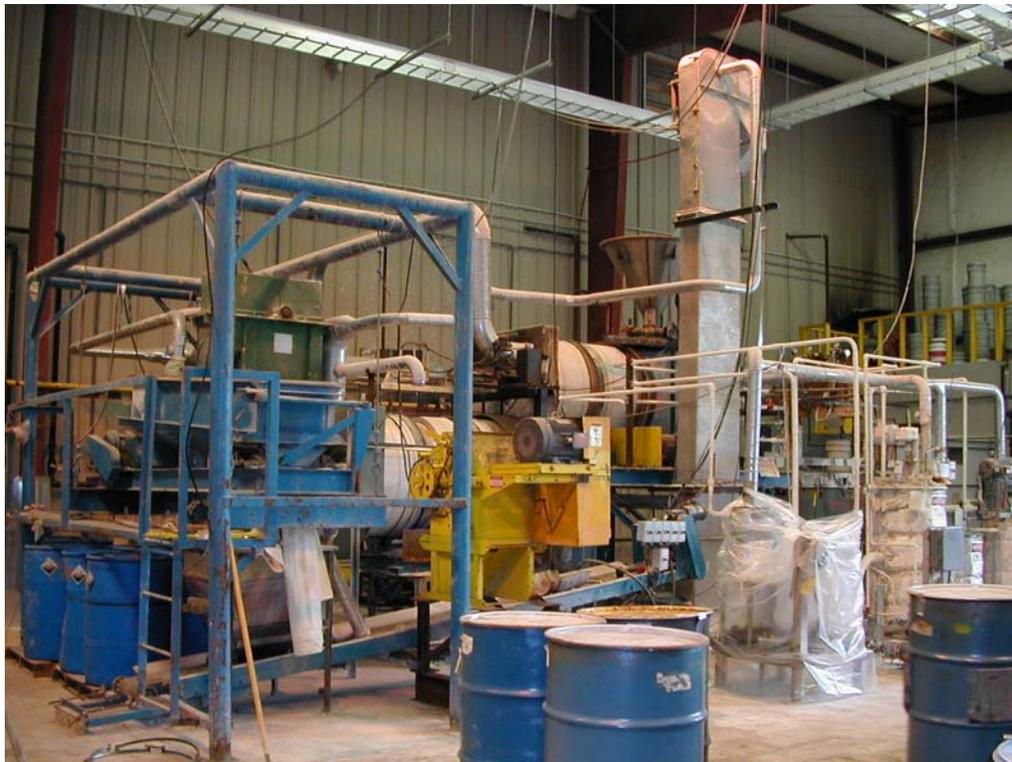
Figure 2. ACT 300 lb per hour NPK granulation pilot plant.
